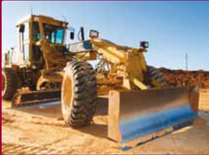
BULLDOZER Hardox 450/500/550 in the blade of the bulldozer.
