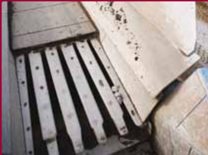
BUCKET Hardox 450/500/550 in the entire bucket or cutting edge and sides depending on the wear situation.
