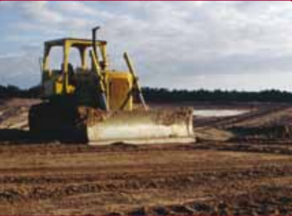
BULLDOZER Hardox 450/500/550 in the blade of the bulldozer.
