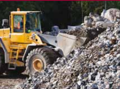
EXCAVATOR BUCKET Hardox 450/500/550 in the excavator bucket. Hardox may be used in the entire bucket or just in the cutting edge and sides depending on the wear situation.
