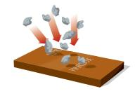
In impact wear, the aggregate rocks hit the surface of the wear component at various anales. A harder grade of Hardox will deliver a longer service life here as well.
