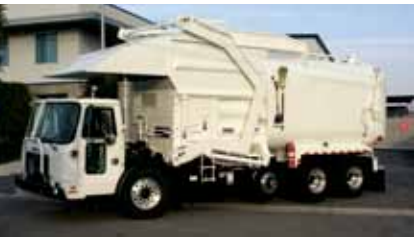
1. GARBAGE TRUCK Hardox 400 or 450. With the increased hardness of Hardox, lighter trucks with higher payloads can be produced. For packer blades inside garbage trucks, Hardox 450 or 500 is used.
