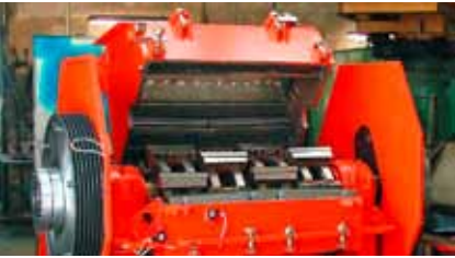
6. PRISMATIC KNIVES Hardox Extreme or 600. For the fragmentation of waste, especially plastics, tires, cables and rubber waste, Hardox can be used. The high toughness of Hardox steels provides substantially higher resistance against chipping.
