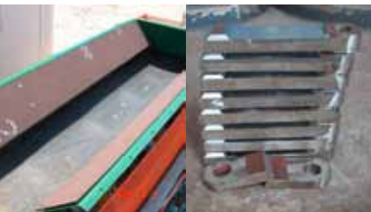
9. CONVEYOR BELT Hardox 450 or 500. Hardox plates can be used to line conveyor belts and be used in moving chains.
