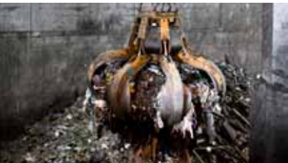
3. GRAPPLES Hardox 450 or 500. Hardox can significantly increase the life of the grapple and other gripping equipment.
