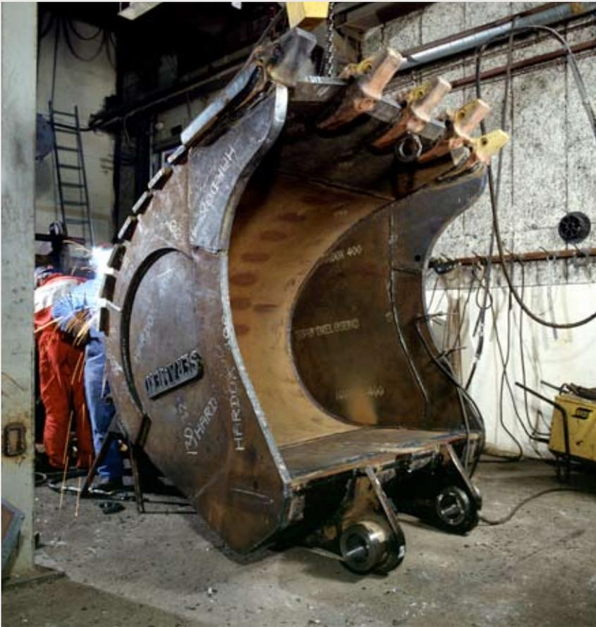
HARDOX HiTuf can be welded with all conventional welding methods available.
