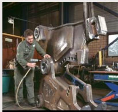
Demolition tools is a typical application where HARDOX HiTuf excellent performance is utilised.
