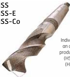
Individual holes can be drilled with an ordinary HSS drill. For rational production, either a micro-alloyed (HSS-E) drill or a cobalt-alloyed (HSS-Co) drill is recommended.
