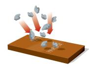
In impact wear, the aggregate rocks hit the surface of the wear component at various angles. A harder grade of Hardox will deliver a longer service life here as well.
