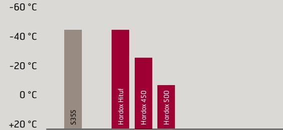
The toughness values for Hardox HiTuf, 450 and 500 are guaranteed minimum values at -40°C, -20°C and 0°C respectively. Compared to a standard S355 steel, Hardox HiTuf for example has about three times higher resistance to permanent deformation (hardness) and an equal resistance to cracking (toughness).
