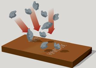
Toughness is the other strong point of Hardox. When hardness makes it wear resistant and strong, toughness is what makes it possible for Hardox to be bent, formed and welded without cracking. If a Hardox wear plate is stressed beyond its yield point and plastically deformed—on purpose in the workshop or when hit by a heavy rock on site—it will resist cracking and if a localized crack should occur it will resist propagation.
