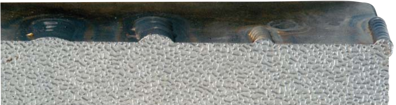
Welded and textured Toolox.
