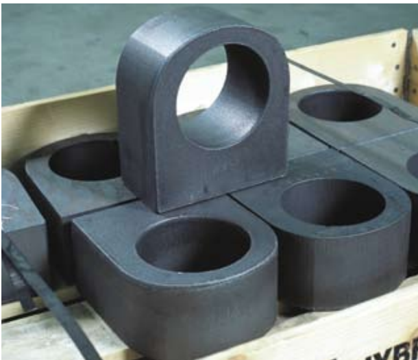
Flame cut blanks for a bearing house.
